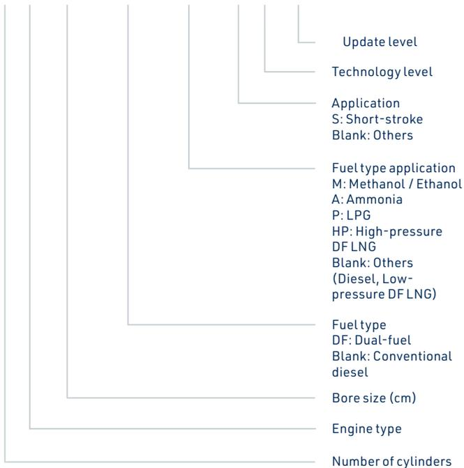
Example engine designation 6X52DF-A-S1.0 representing a WinGD 6 cylinder, short-stroke engine for dual-fuel operation with ammonia and diesel.
