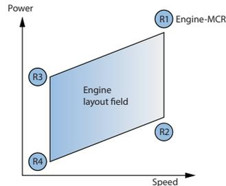
Any power and speed within the respective engine layout field may be selected as the Contracted-MCR (CMCR) point for an engine.
