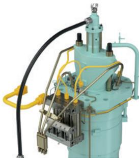
engine is running in diesel mode and to inject a small amount of pilot fuel in methanol/ethanol mode. The pilot fuel injection is required to have an accurate ignition of the methanol fuel at all engine loads.
