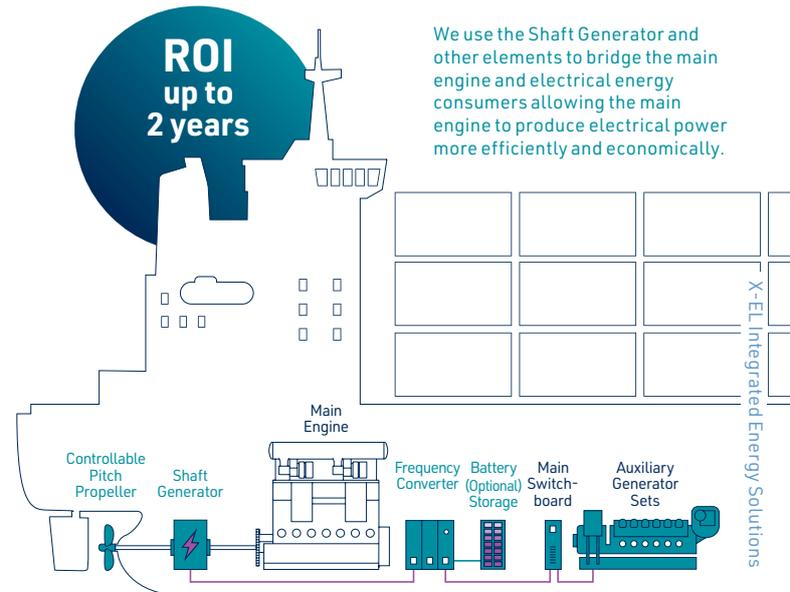
We use the Shaft Generator and other elements to bridge the main engine and electrical energy consumers allowing the main engine to produce electrical power more efficiently and economically.
